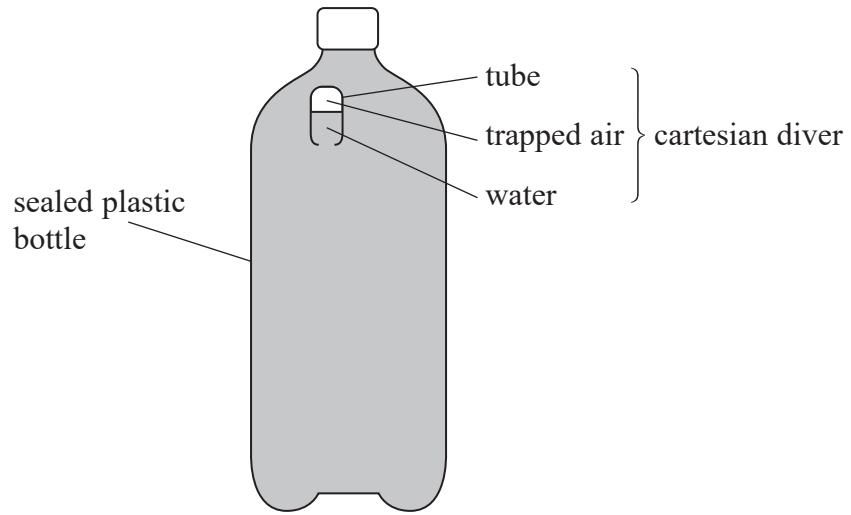
The student squeezes the bottle. More water is forced into the tube, and the volume of the trapped air decreases.
